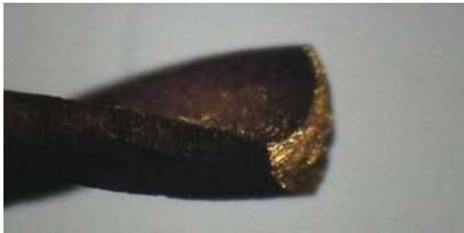
Fig 20. Machine vision image of DLC coated drill bits
