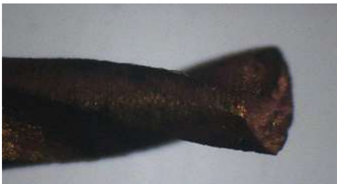
Fig 21. Machine vision image of DLC-Ti coated drill bits
