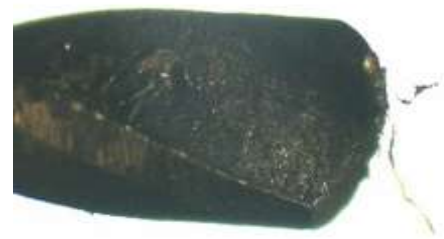
Fig 20. Machine vision image of DLC coated drill bits
