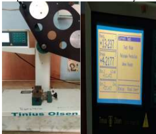
Figure 15. Impact Test Results for Double Layer Roselle Fiber with Filler
