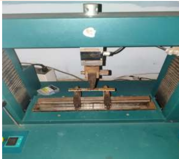
Figure 18. Flexural Test Results for Double Layer Roselle Fiber
