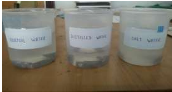
Figure 10. Specimens Soaked in Water (3 different waters) for Water Absorption Test
