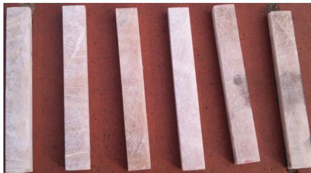
Fig: 2 Test Composite Specimen E-Glasses, Aloevera &Polyester Resin
