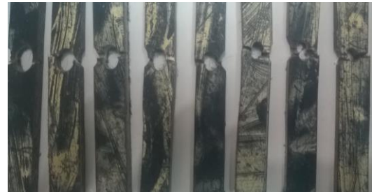
Figure.6. Typical open hole after impact specimen
