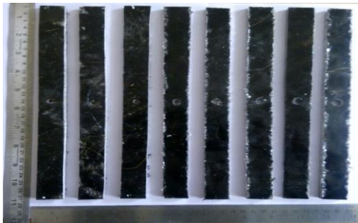
Figure.3. Typical open hole before tensile specimen
