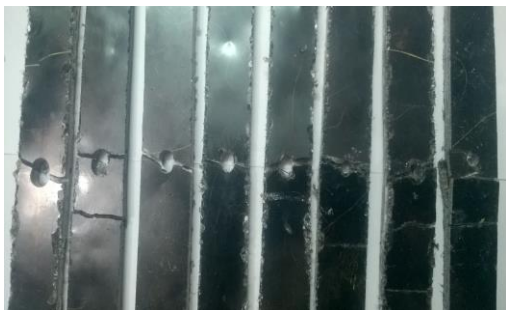
Figure.4. Typical open hole before tensile specimen
