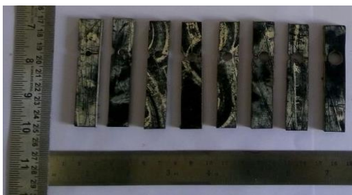
Figure.5. Typical open hole before impact specimen
