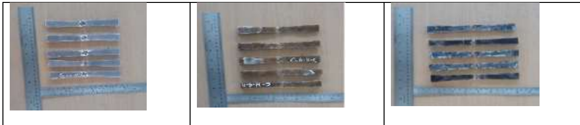
Fig:6 Specimens of open hole tensile strength after drill
