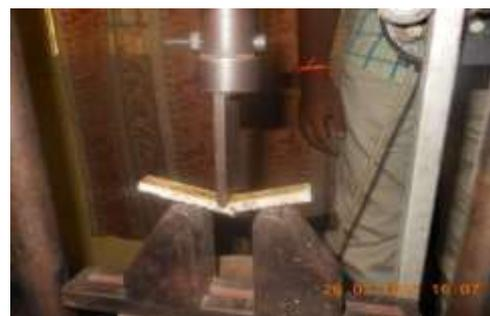
Fig. 4. UTM machine Sample loaded condition for Flexural testing.
