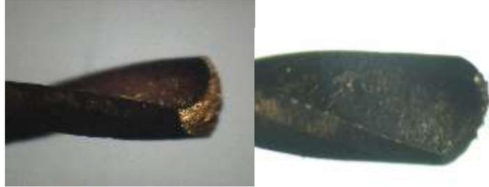
**Figure 9 (a) mission vision image of DLC coated drill bits**
