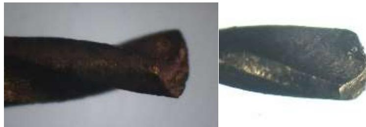
**Figure 9(b) mission vision image of DLC-Ti coated drill bits**
