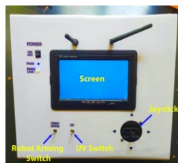
Fig. 1 Ground station controller
