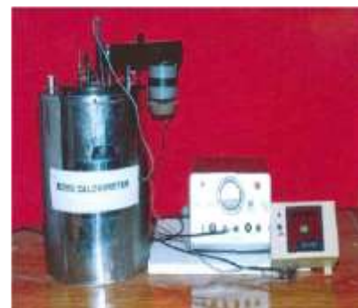
Fig 2.8 Instrument of bomb calorimeter
