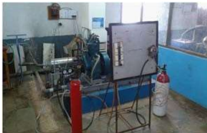
Figure 1 Dual fuel engine with CNG/Hydrogen induction arrangement
