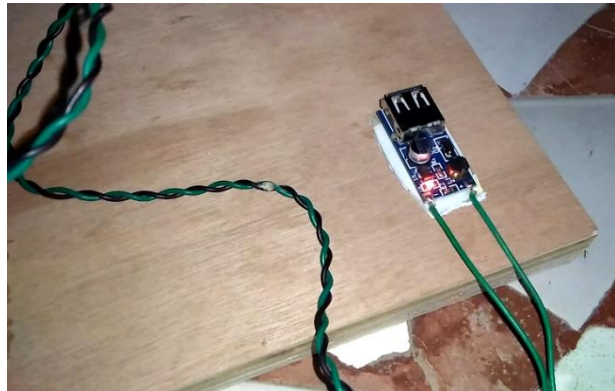
Figure 5 Output LED blinking in the Boost converter
