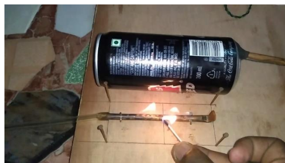
Figure 6 Lighting of the Biogas in the burner
