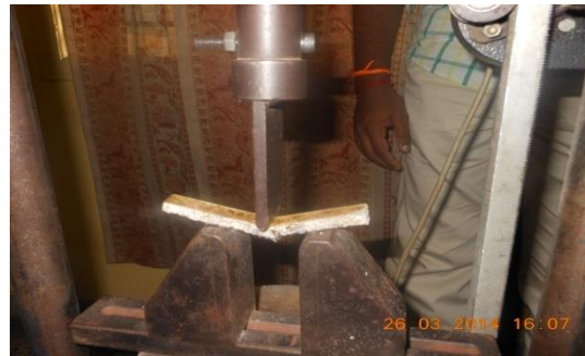
Fig. 4. UTM machine Sample loaded condition for Flexural testing.
