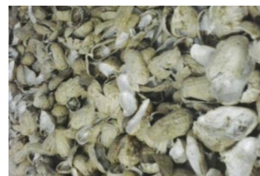
(b) Groundnut shell fiber used for making composite.
