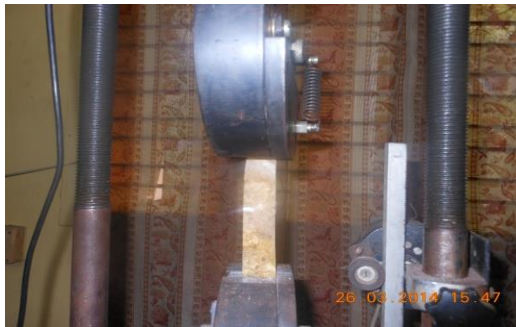
Fig. 3. UTM machine Sample loaded condition for tensile testing
