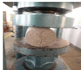
Fig 2. split tensile strength of concrete
