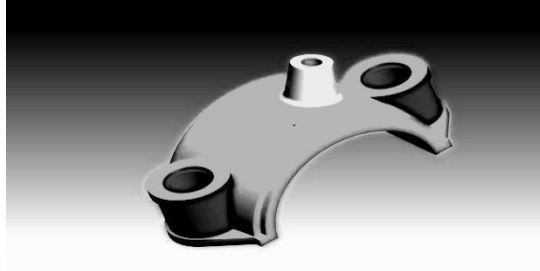
Fig. 4.2 Cover for connecting rod
