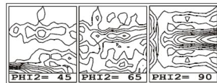
Fig 3.2: X-ray ODFs of type 316L stainless steel (80% reduction)
