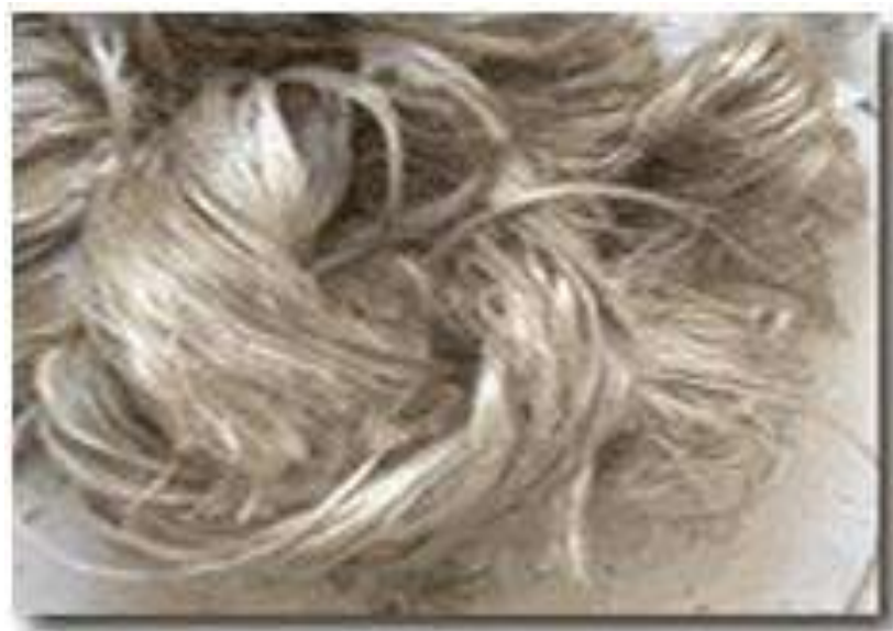
Fig 2.1 Jute fiber obtained from stem of Jute plant (Muthuvel et al (2013)).
