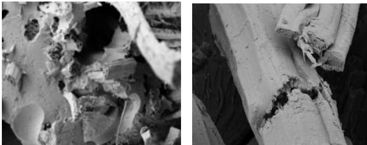
Fig 4.1 SEM micrographs showing details of the fractured surface of aged pultruded composites.
