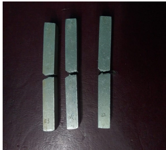
Fig 8. AMMC material after impact test
