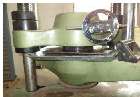
Figure 7: Placing the material in UTM
