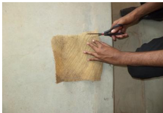
Figure 3: Cutting Coir Sheath
