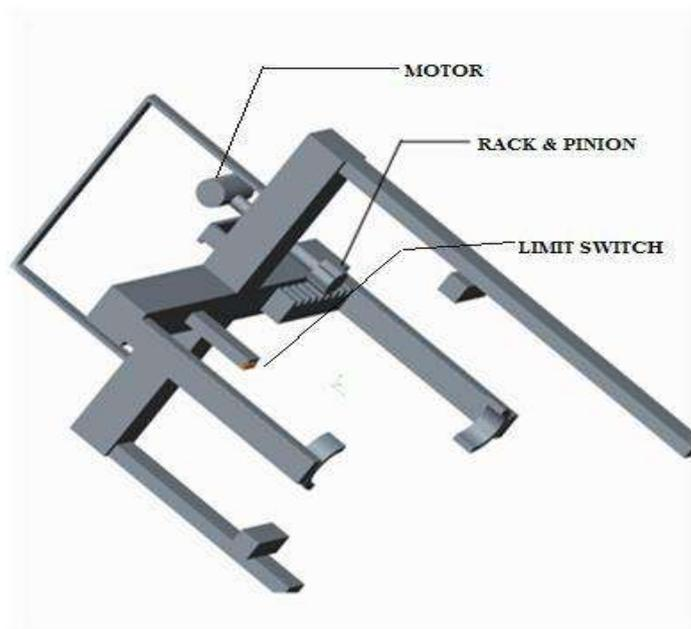
Fig.1 CAD model of rescue robot
